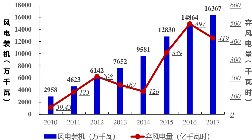
Wind Power Installation and Abandoned Wind Power in Recent Years
