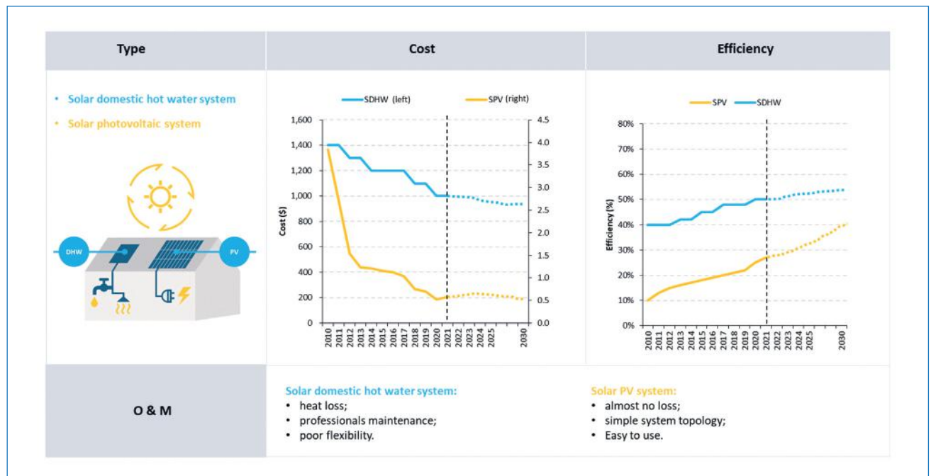
Fig. 2.4. Comparison of solar domestic hot water system and photovoltaic system. Provided by Tsinghua University with Permission for Reproduction.
