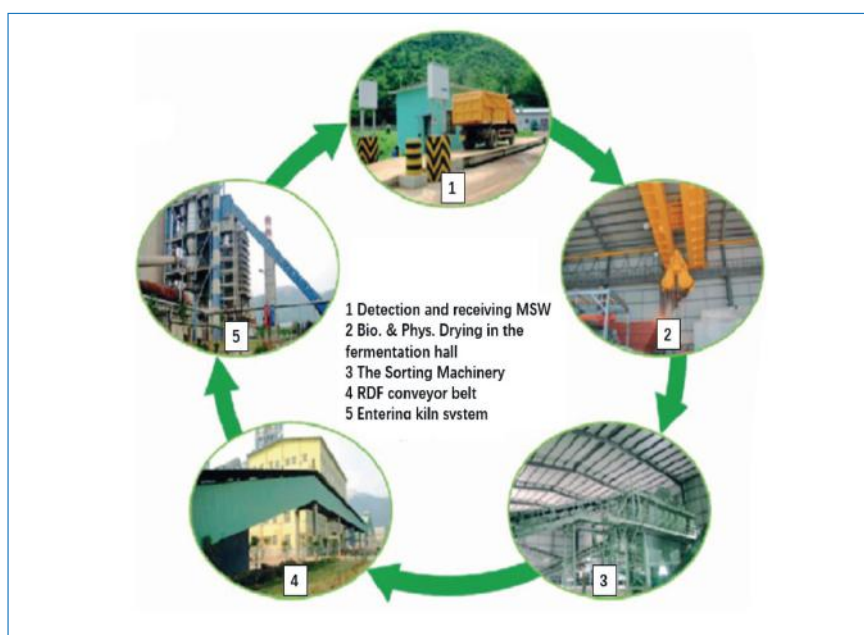
Fig. 5.38 Domestic waste disposal flow chart of cement kiln 69
