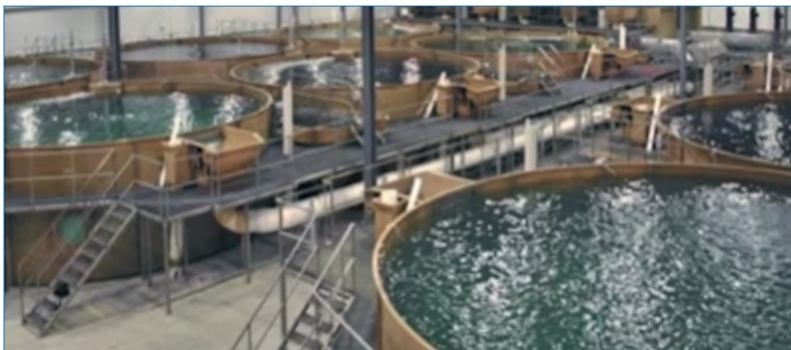
Fig. 1.15. Indoor recirculating aquaculture system
